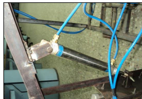
Fig. 7 : Cylinder For Rocker-Front/Rear
