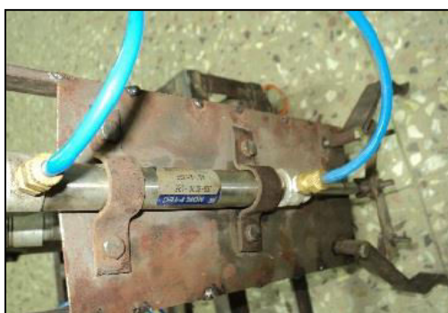
Fig. 9 : Cylinder For Gripper
