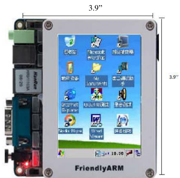
Fig.1: Friendly ARM with running Win CE Operating system
